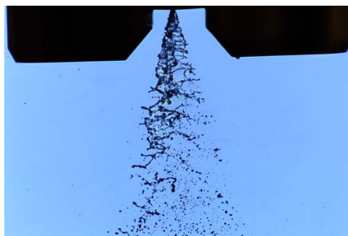
Figure 1: Example of a liquid jet discharged from a compound nozzle (from Triballier et al [4])
